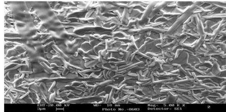
3b. SEM  $\text{La}_{0.5}\text{Bi}_{3.5}\text{Ti}_3\text{O}_{12}$  at 5x
