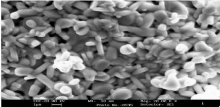
3c. SEM  $\text{La}_{0.1}\text{Bi}_{3.9}\text{Ti}_3\text{O}_{12}$  at 20x
