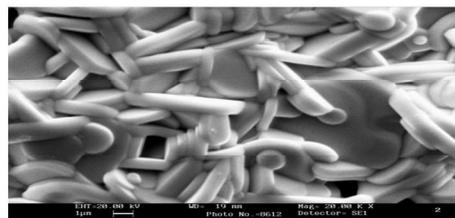
3d. SEM  $\text{La}_{0.5}\text{Bi}_{3.5}\text{Ti}_3\text{O}_{12}$  at 20x
