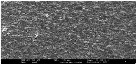
3a. SEM  $\text{La}_{0.1}\text{Bi}_{3.9}\text{Ti}_3\text{O}_{12}$  at 5x
