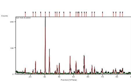
XRD of  $\text{La}_{0.1}\text{Bi}_{3.9}\text{Ti}_3\text{O}_{12}$
