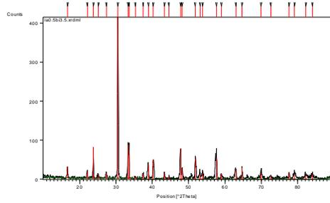
XRD of  $\text{La}_{0.5}\text{Bi}_{3.5}\text{Ti}_3\text{O}_{12}$
