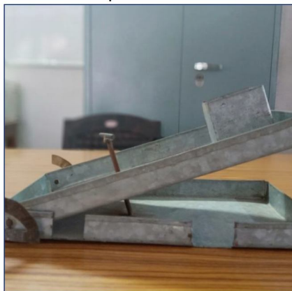
Fig. 2 Apparatus for measuring Coefficient of static friction
