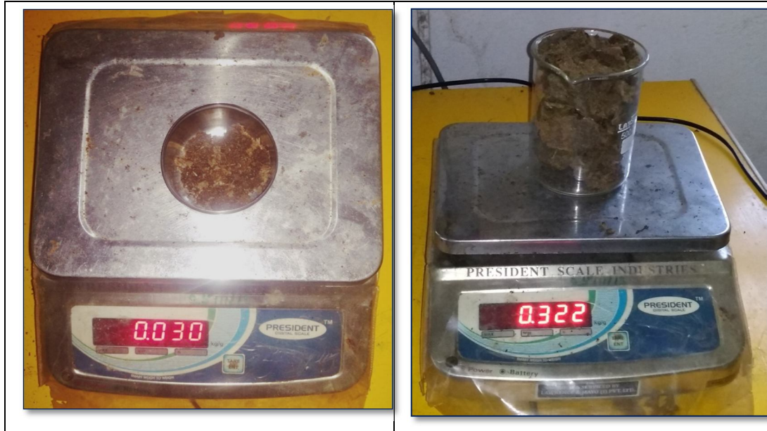
Fig. 1 Apparatus for measuring moisture content and bulk density
