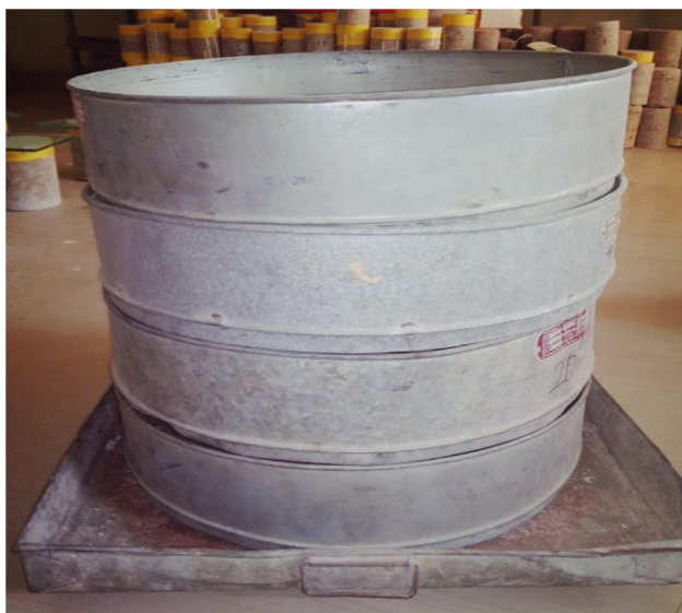
Fig. 3 Apparatus for measuring the sieve analysis
