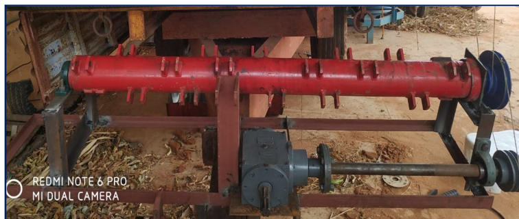
Fig. 5 Beating roller mounted on the main frame
