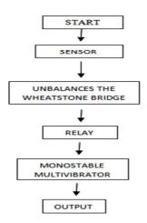
WEIGH IN MOTION: The process of dynamic weighing consists in recording and processing signals generated in sensors under the influence of the axle loads of a moving vehicle. Since the sensors are embedded in pavement perpendicularly to the direction of motion, each vehicle passing over the WIM site is weighed
