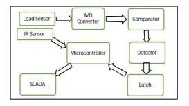
SCADA VIEW OF PROPOSED PARAMETERS: The three sensors IR sensor, strain gauge sensor (load cell) are complied to all the parameters. (WIM, Speed detector, TSC) in accordance with the circuit diagram after the process the SCADA detector shows real time recording and transmitted to control soon and further the recorder recognize the plate number through license plate detection.
